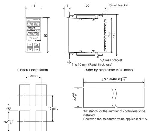
Normal Allowable Deviation= $\pm$  (Value of JIS B 0401-1999 tolerance grade IT18) /2
